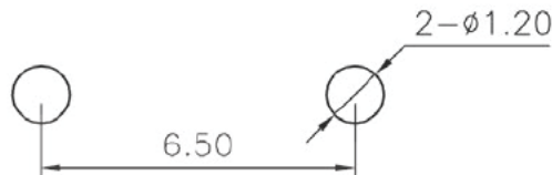
PCB Layout (Pattern Side)
